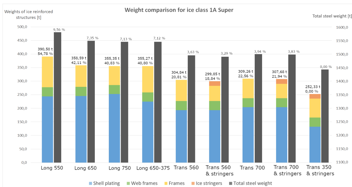
Figure 28: Weight results for ice class IA Super. Weight increase percentiles from the lightweight option are written above weights of ice reinforced structures and the total steel weight correspondingly.
