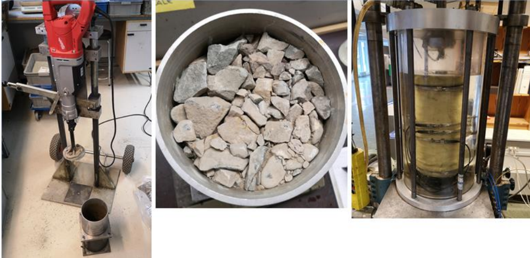
Figure 15: From left to right: Compaction apparatus and mould; compacted test specimen; triaxial cell being filled with water
