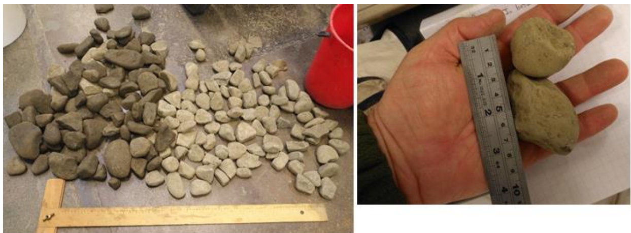
Figure 10: Larger granular fraction of the sample with a 1-m ruler (left hand side) and smaller granular fraction with a 30cm ruler (right hand side)
