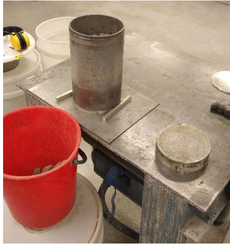
Figure 3: Placement of rocks in the cylinder
