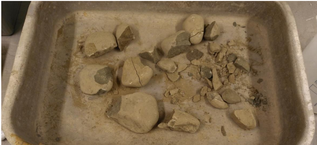
Figure 5 : Example of highly damaged/crushed material
