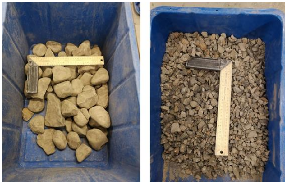
Figure 21: 50-150mm natural material to gravel (after 2 crushing cycles)
