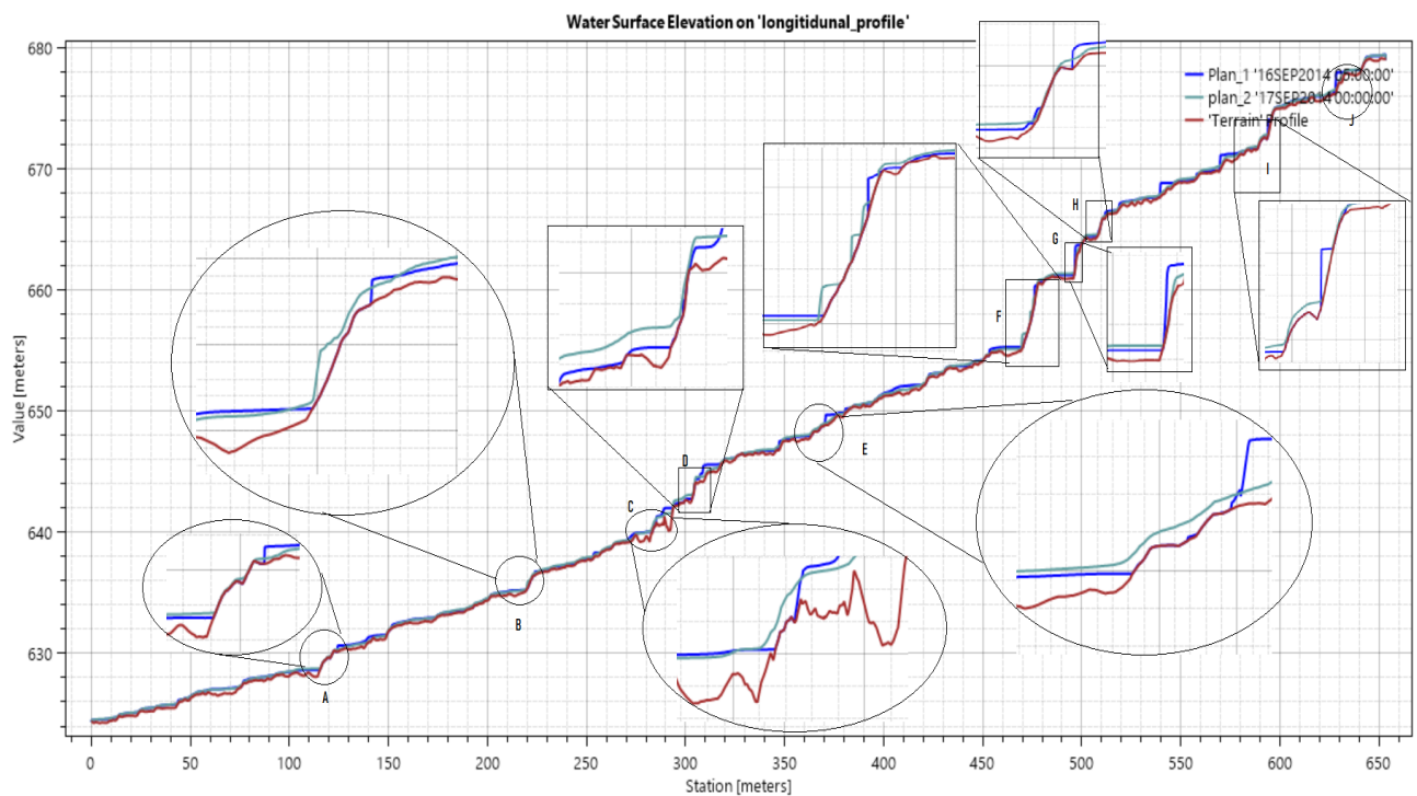
Figure 6-31: Longitudinal water depth profile along river centerline (longitudinal profile); blue colored line represents simulation 1's (5-hr simulation time) water depth; and the dark green colored line represents the simulation 2's water depth (24-hr simulation).
