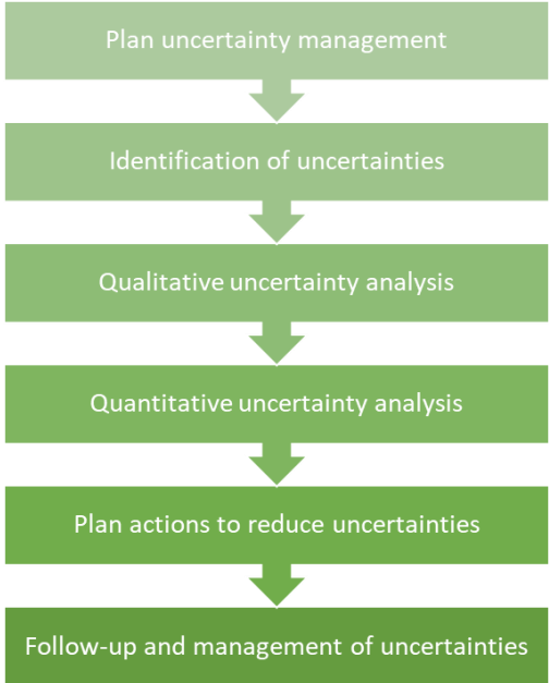
Figure 6 Illustration of PMI's six step model for analysis and management of uncertainties
