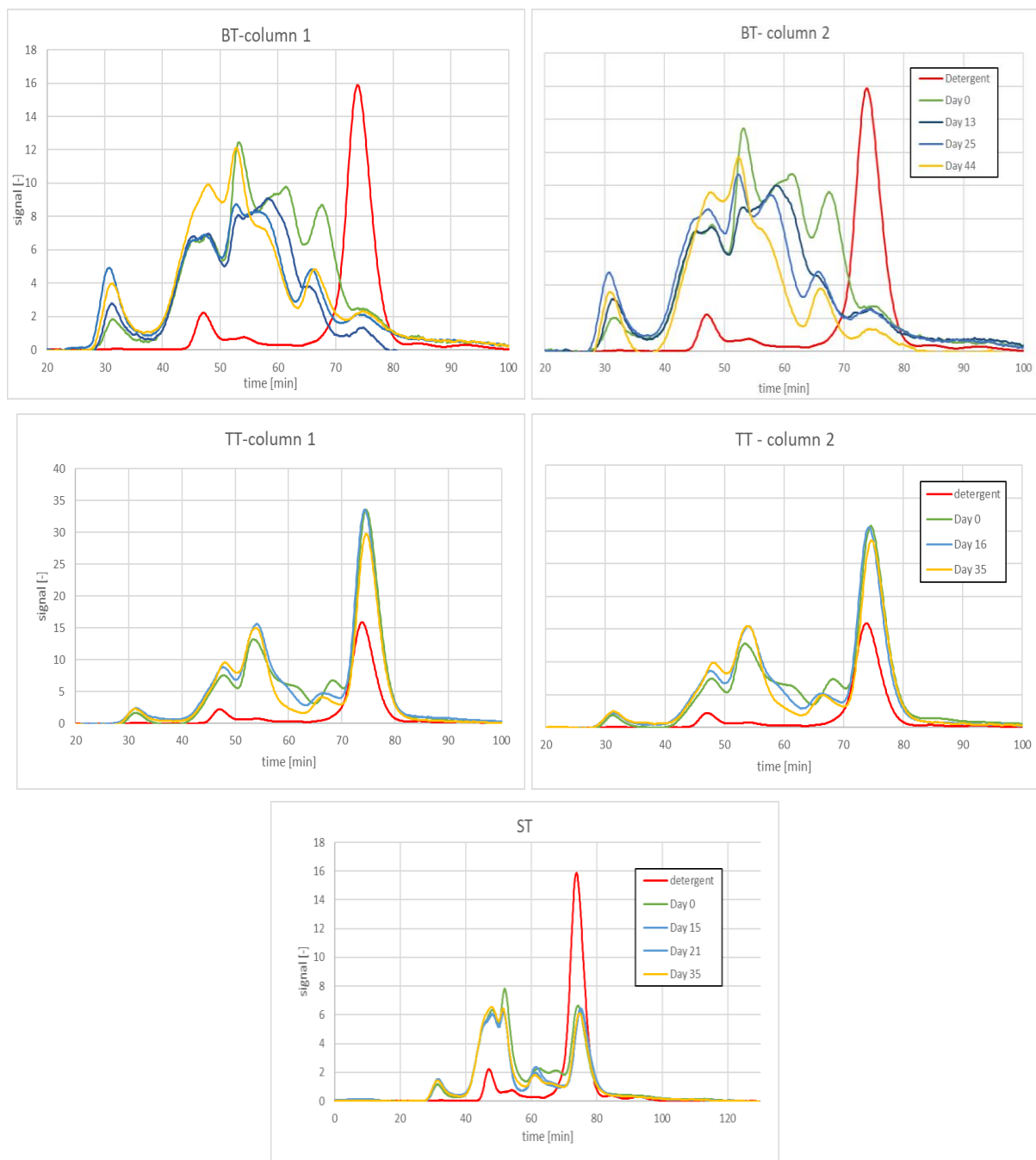
Figure 3.10: Chromatograms for the BT, ST and TT samples, showing the OCD-graphs. The detergent represented here was diluted with a factor of 500.
