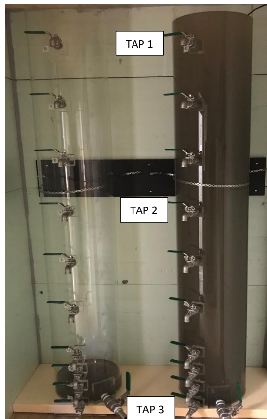
Figure 2.1: A picture of the columns used in the lab setup. Tap 1, 2 and 3 were used in the present experiments. Each column had a height of 2 meters and a diameter of 30 cm. Tap 1 was initially 25 cm under the water surface. Tap 3 was 1 cm above the bottom.
