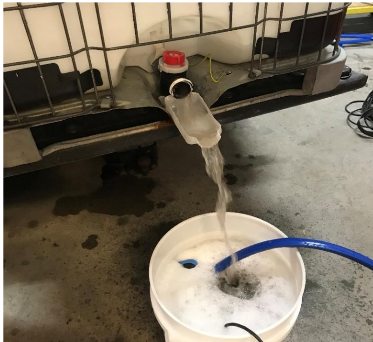
Figure 2: The water from Smestadtunnelen (ST) was transferred to the columns by pouring the water into the bucket, then using a submersible pump to pump the water into the columns. For the other tunnels smaller containers were used for the transportation. These were shaken before also using the bucket and the submersible pump to transfer the water into the columns.
