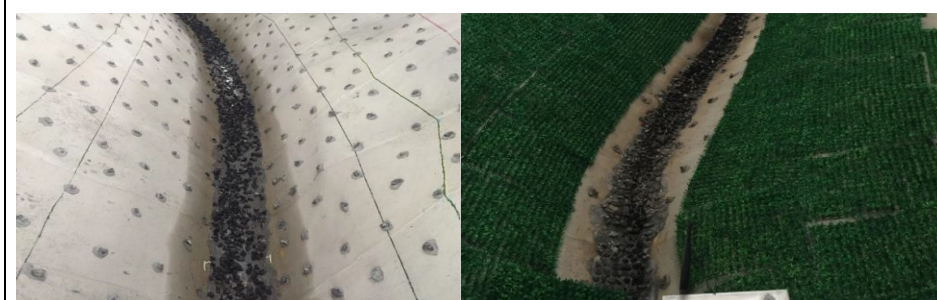
Figure 4.12 River banks roughened with blocks and plastic straw mat (Adapted from report ANNEX H-3)
