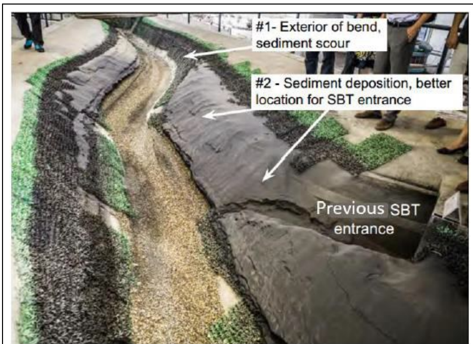
Figure 4.11 Initial SBT and modified SBT location (#2) (Adapted from report ANNEX H-3)
