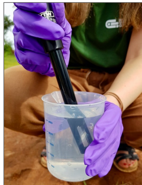
Figure 19: Conductivity measurement with IDS sensor
