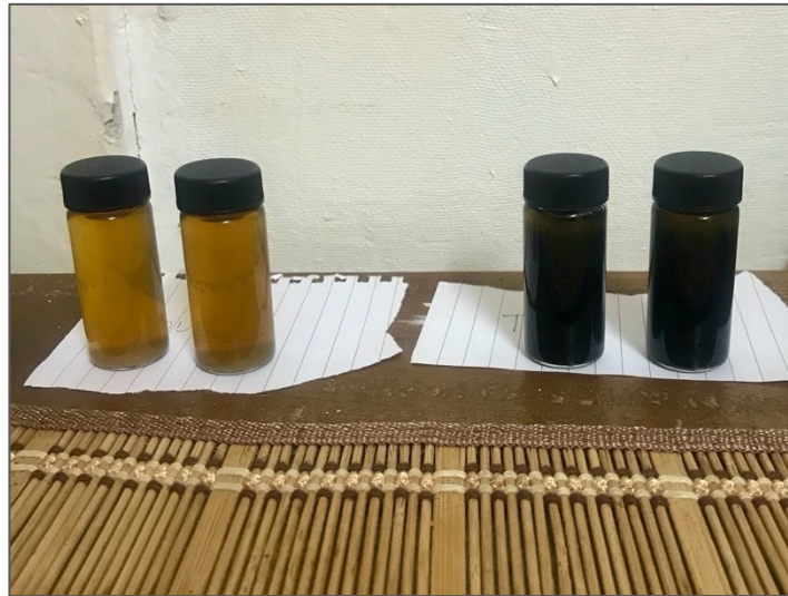
Figure 22: H 2 S-test, two negative test samples (left) and two positive test samples (right)
