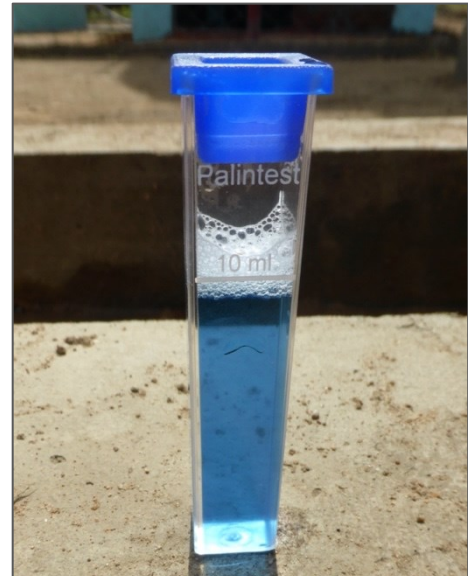
Figure 18: Test tube containing water sample and a dissolved alkavis tablet
