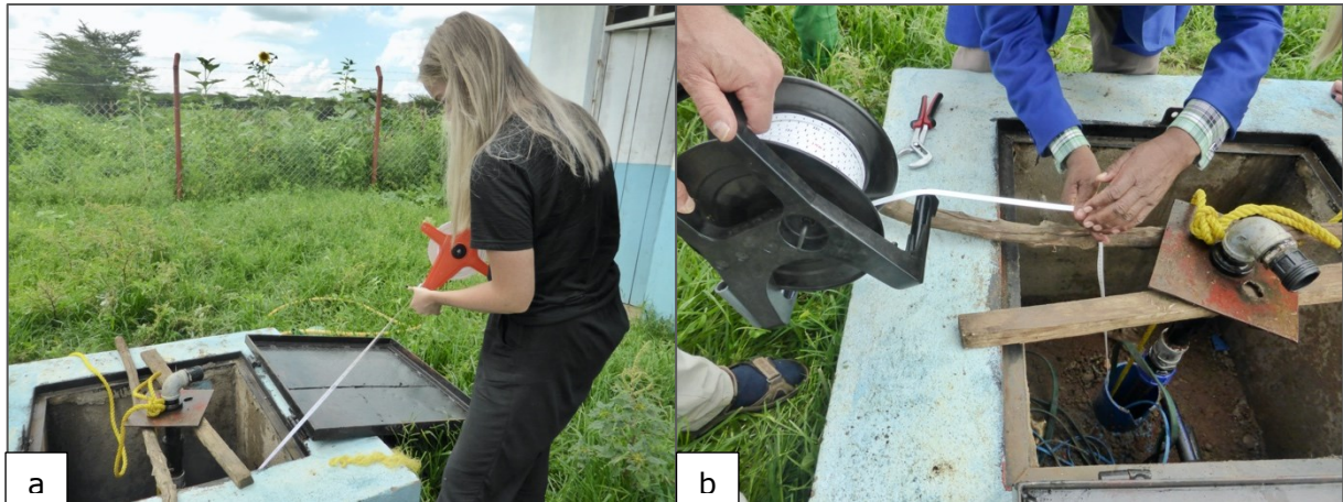
Figure 14: Water level measurement with a) The Pocket Dipper and b) KLL-Light Electric Contact Meter
