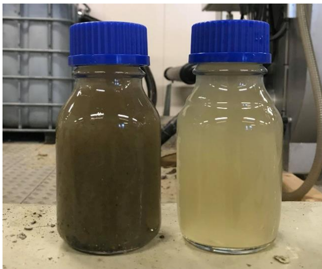
Figure 3.12 Sludge samples from microsieve (left) and membrane tank(right).
