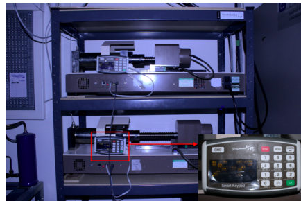
Figure 4.5: Cell pressure piston (bottom) and back pressure piston (top) is regulated from panels or GDSLAB software.
