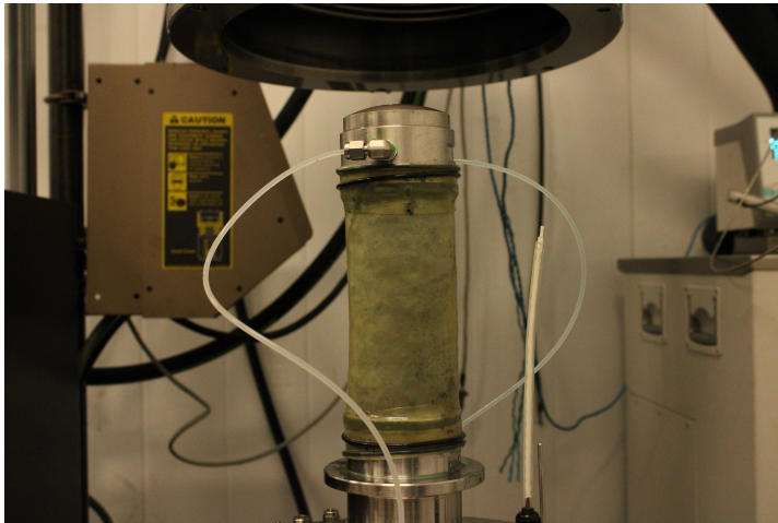
Figure 4.6: Sample with membrane and o-rings.
