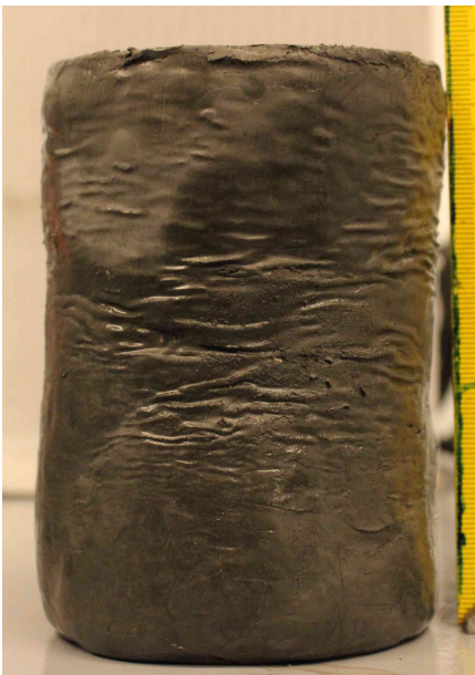
Figure 4.15: Cylindrical deformation mode.
