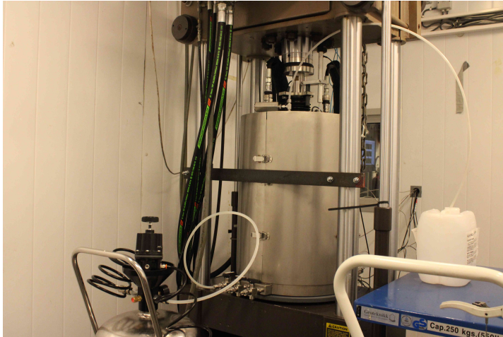
Figure 4.7: Set up for filling the cell with oil.
