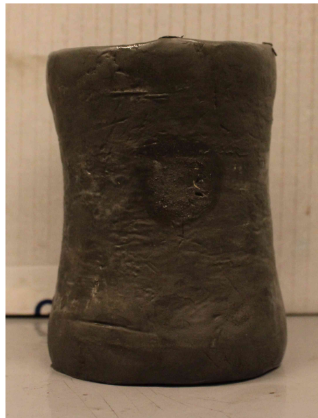
Figure 4.16: Hourglass deformation mode.
