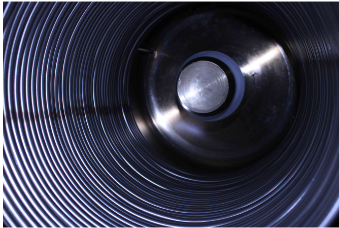
Figure 4.2: Coil system inside the triaxial cell.
