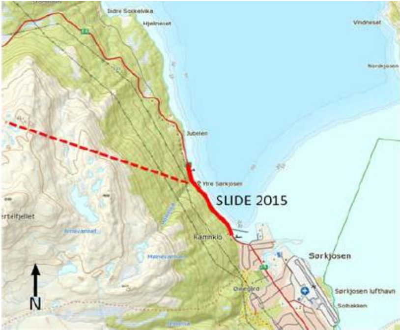
Figure 18: The 2015 slide sent the shoreline marked by a solid line into the fjord. The dotted line was a rock tunnel under construction.
