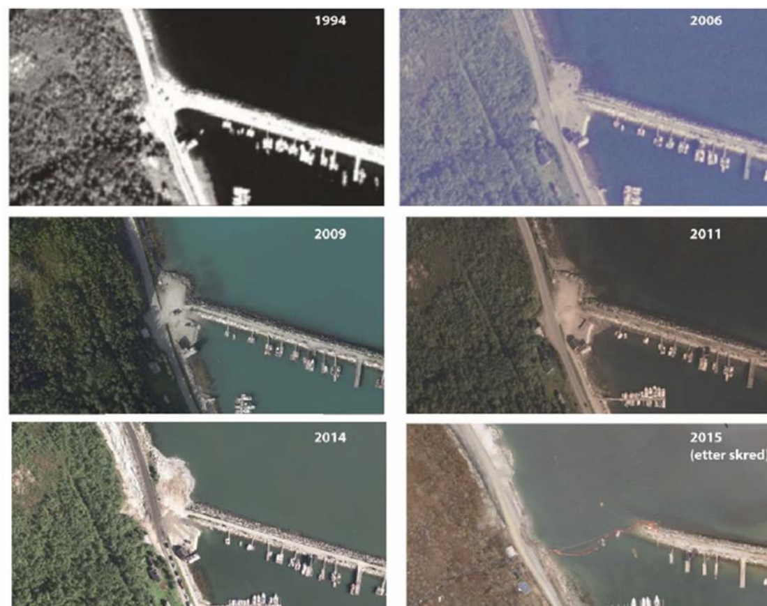
Figure 29: Orthophotos of the pier at Sørkjosen in the period 1994-2015 illustrate filling in over time, as well as the situation after the slide. (Nordal.S, L'Heureux.J, Skotheim. A, 2016)
