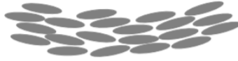
Figure 1: The figure illustrates the orientational ordering within a nematic liquid crystal. The elongated molecules tend to align their long axes, while flowing like a liquid, but there is no positional correlation between the molecules.
