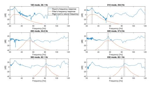
**Figure 4.15:** Frequency responses of modes in room A. The black dashed lines marks theoretical natural frequencies with rigid surfaces and the black solid lines marks their actual locations in the real room.
