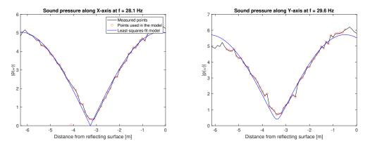
**Figure 4.7:** Measured and modelled standing wave, mode (1,0,0) and (0,1,0) in room A.
