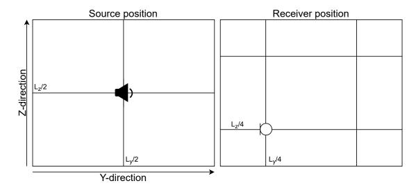
**Figure 2.3:** Position of source and receiver at intersection between nodal lines for a  $(n_x, 1, 1)$  mode (left), and a  $(n_x, 2, 2)$  mode (right).
