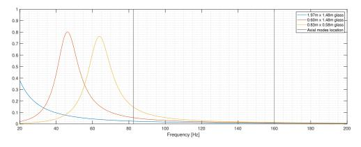
**Figure 4.25:** Estimation of absorption coefficient for 6.36 mm thick glass wall segment in room B.
