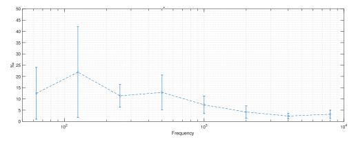
**Figure A.5:** Degree of non-linear decay,  $\xi$ , for T20 in room B.
