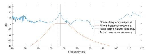
**Figure 3.10:** Example of how the frequency response of a measurement of a single mode looks, and the frequency response of the filter designed to completely isolate it.
