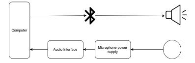
Figure 3.3: Block diagram of how the measurement equipment is connected.
