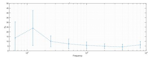
**Figure A.2:** Degree of non-linear decay,  $\xi$ , for T20 in room A.
