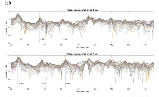
**Figure 4.4:** Frequency response along X- and Y-axis of room A. The black dashed lines marks theoretical natural frequencies with rigid surfaces and the black solid line marks their actual locations in the real room.
