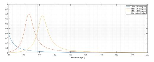
**Figure 4.24:** Estimation of absorption coefficient for 8.36 mm thick glass wall segment in room A.
