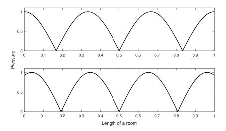
**Figure 1.1:** Example of how a purely imaginary impedance can shift the phase of the reflected wave.
