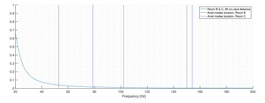
**Figure 4.23:** Estimation of absorption coefficient for 25 mm thick, 90 cm wide and 270 cm tall gypsum wall segment in rooms B and C.
