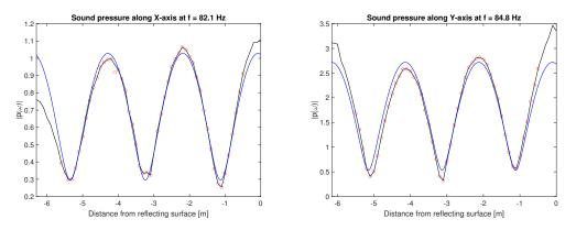
**Figure 4.9:** Measured and modelled standing wave, mode (3,0,0) and (0,3,0) in room A.
