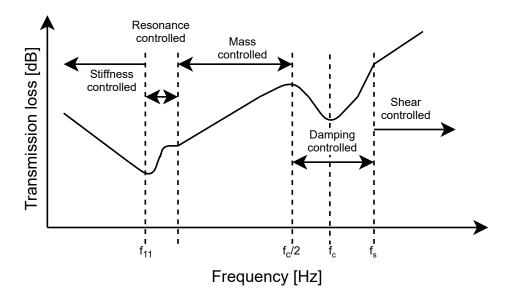
**Figure 2.1:** Transmission loss versus frequency for a thin panel. Figure inspired by Figure 9.15 in [10].
