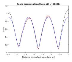
Figure 4.12: Measured and modelled standing wave, mode (3,0,0) in room B.
