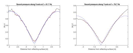
**Figure 4.13:** Measured and modelled standing wave, mode (1,0,0) and (0,1,0) in room C.
