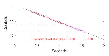
Figure 2.8: Decay curve with evaluation range for T20 and T30
