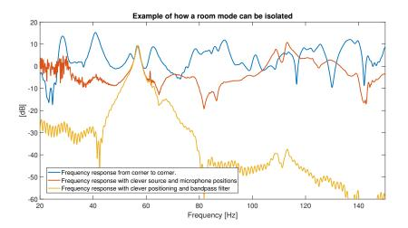
**Figure 2.4:** Example of how a room mode can be isolated through source and receiver positioning as well as bandpass filtering.
