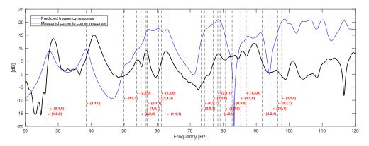
**Figure 4.1:** Global frequency response measured and predicted frequency response in room A, measured from corner to corner.
