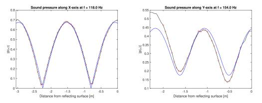
**Figure 4.14:** Measured and modelled standing wave, mode (2,0,0) and (0,2,0) in room C.
