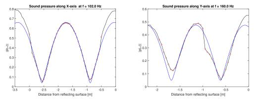
**Figure 4.11:** Measured and modelled standing wave, mode (2,0,0) and (0,2,0) in room B.
