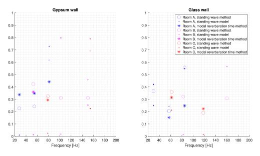
**Figure 4.21:** Absorption coefficients estimated through the different methods. Data points that meets the quality criteria are enlarged.
