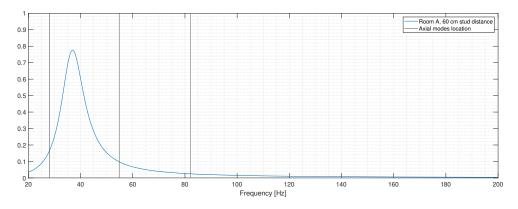
**Figure 4.22:** Estimation of absorption coefficient for 25 mm thick, 60 cm wide and 270 cm tall gypsum wall segment in room A.
