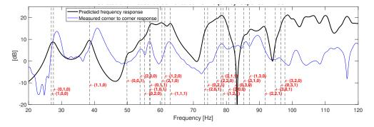
**Figure 3.2:** Predicted natural frequencies and frequency response compared to the measured corner to corner frequency response. The impact the loudspeaker has on the measured response have been reduced through division in the frequency domain.
