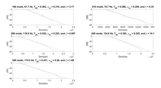
**Figure 4.20:** Decay curve, modal reverberation time, mean absorption coefficient and linearity ratio of normal modes in room C.
