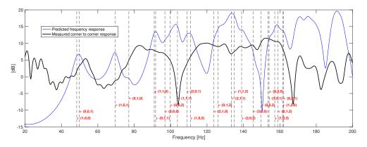
**Figure 4.2:** Global frequency response measured and predicted frequency response in room B, measured from corner to corner.
