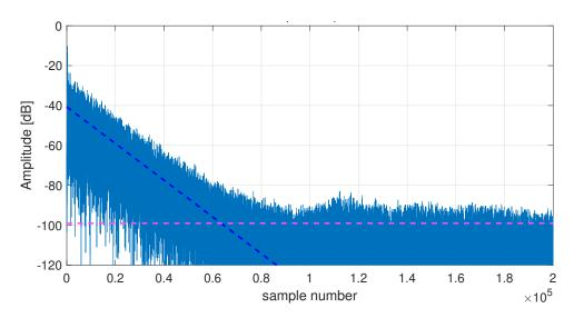
**Figure 2.6:** A filtered impulse response where the slope of the squared impulse response is illustrated by the dashed blue line, and the mean background noise level is illustrated by the pink line.
