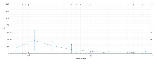
Figure A.6: Curvature of the decay rate in room B.
