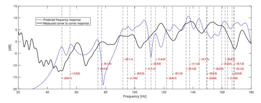
**Figure 4.3:** Global frequency response measured and predicted frequency response in room C, measured from corner to corner.
