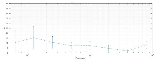
**Figure A.8:** Degree of non-linear decay,  $\xi$ , for T20 in room C.
