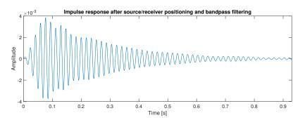
Figure 2.5: Example of how the impulse response may look after one mode is isolated.
