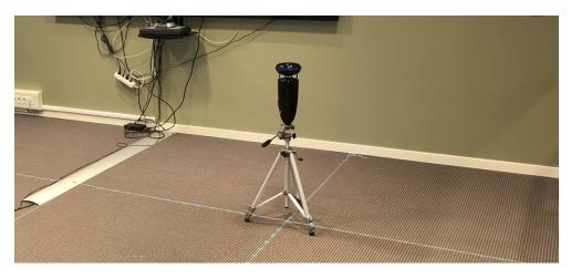
**Figure 3.8:** Source placed on an intersection between three nodal planes, as the acoustic center of the speaker is placed at a fourth of the room's height.
