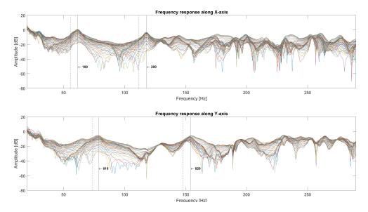
Figure 4.6: Frequency response along X- an Y-axis of room C.
