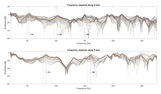
Figure 4.5: Frequency response along X- and Y-axis of room B.
