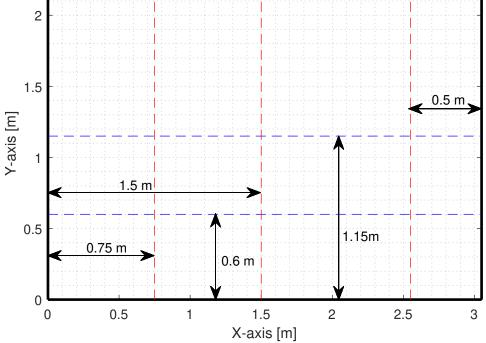
Figure 3.7: Pressure nodes discovered experimentally in room C.
