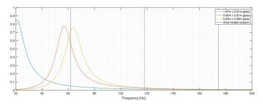
**Figure 4.26:** Estimation of absorption coefficient for 6.36 mm thick glass wall segment in room C.
