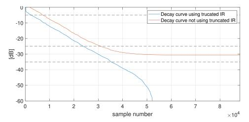
**Figure 2.7:** Decay curve of a backwards integrated impulse response with and without truncation. The dashed lines marks the levels -5, -25 and -35 dB.
