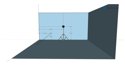
**Figure 3.4:** Illustration of loudspeaker and microphone positions in room A when measuring the standing wave patterns between the wall in x=0 and  $x=L_x$ . The microphone's acoustic center was moved along the black line.
