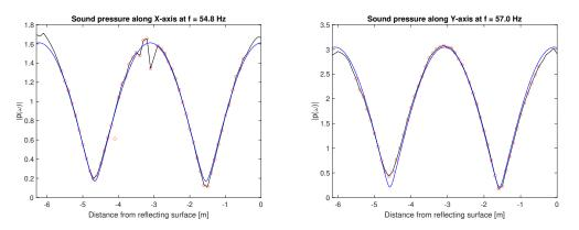
**Figure 4.8:** Measured and modelled standing wave, mode (2,0,0) and (0,2,0) in room A.
