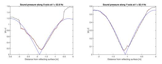
**Figure 4.10:** Measured and modelled standing wave, mode (1,0,0) and (0,1,0) in room B.
