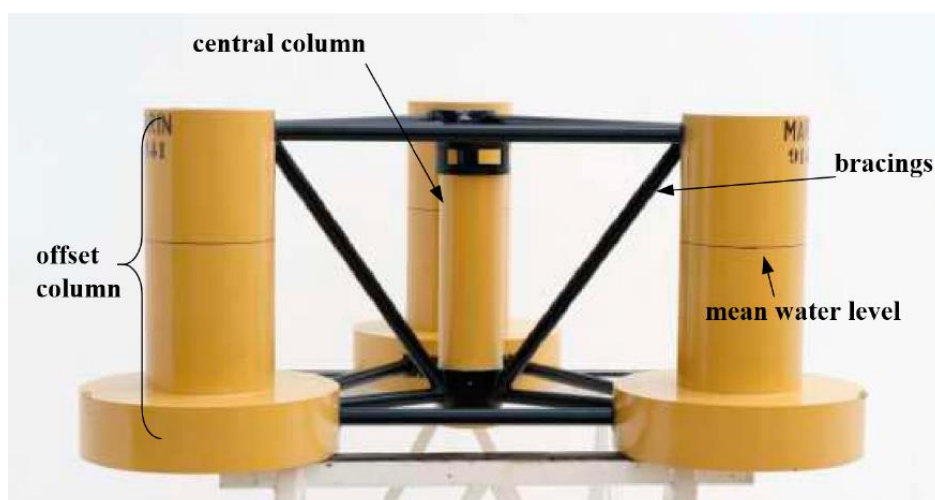
Figure.5. 1/50 scale model of the DeepCwind semi-submersible platform.
