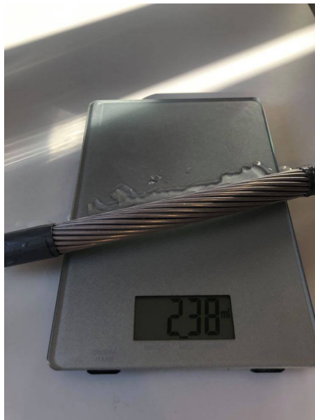
Figure 5.3: Conductor after put into water. Weight: 238g
