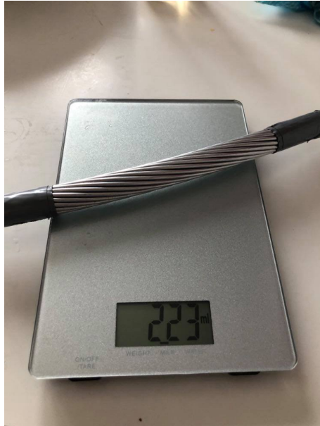
Figure 5.2: Conductor before put into water. Weight: 223g
