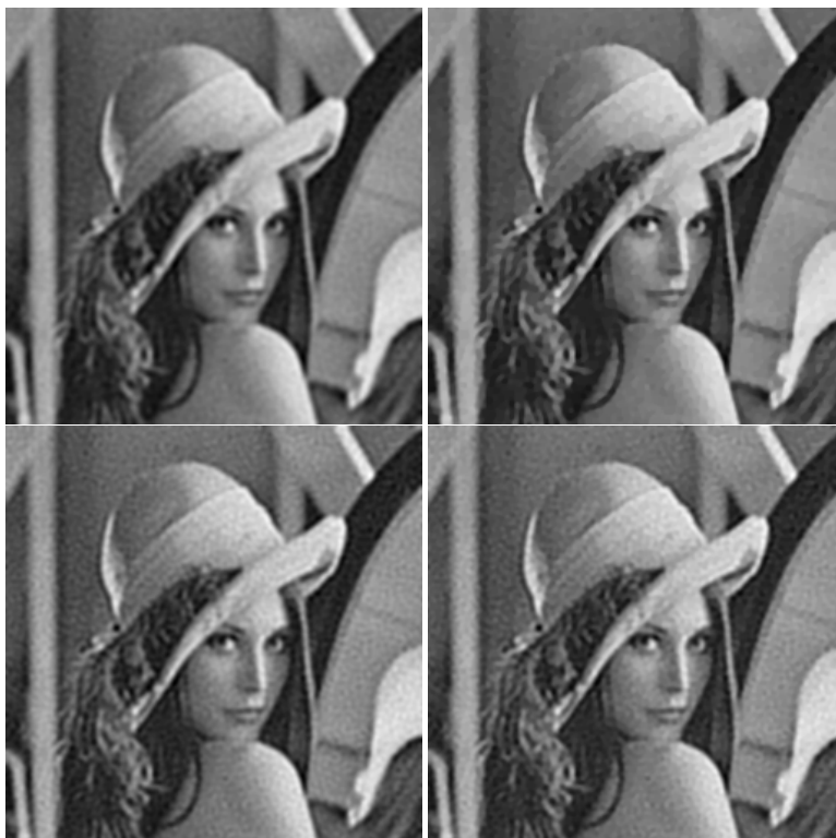
Figure 7.20: Deconvolution results part 2. The upper left image is the QV reconstruction using the quasi optimality criterion. The upper right image is the TV reconstruction using the previous image as the approximate solution. The bottom left image is
