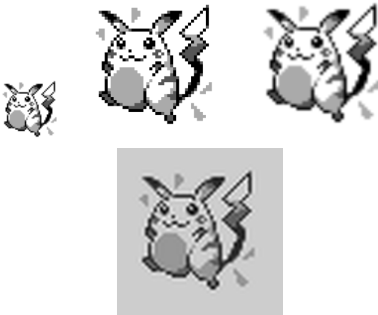
Figure 4.7: Left is a 56 \times 56 image. All other images are upsampled images with \alpha = 2.0 . The upper middle image is created using nearest-neighbour interpolation. The upper right image is created using bilinear interpolation. The bottom image is created using bicubic interpolation.
