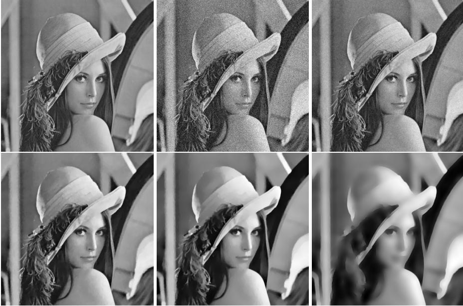
Figure 2.5: Original image u , noisy image v = u + \sigma w with Gaussian noise and \sigma = 0.1 and TV reconstructions using \lambda = 0.01, 0.05, 0.1, 0.5 respectively. Note that parameters differ greatly in size from figure 2.4.
