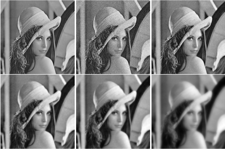
Figure 2.4: Original image u , noisy image v = u + \sigma w with Gaussian noise and \sigma = 0.1 and QV reconstructions using \lambda = 1.0, 5.0, 10.0, 50.0 respectively.
