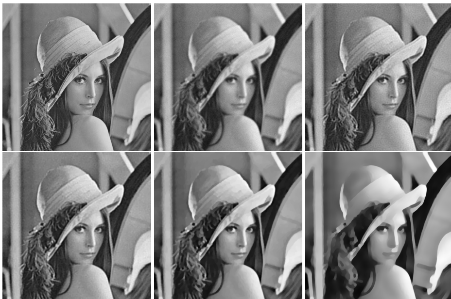
Figure 5.1: Original image u , blurred and noisy image v = Au + \sigma w with \sigma = 0.02 and TV reconstructions using \lambda = 0.0001, 0.001, 0.01, 0.1 respectively. The blur operator A is a Gaussian blur with a 15 \times 15 kernel and \sigma_{\text{blur}} = 1.5 .
