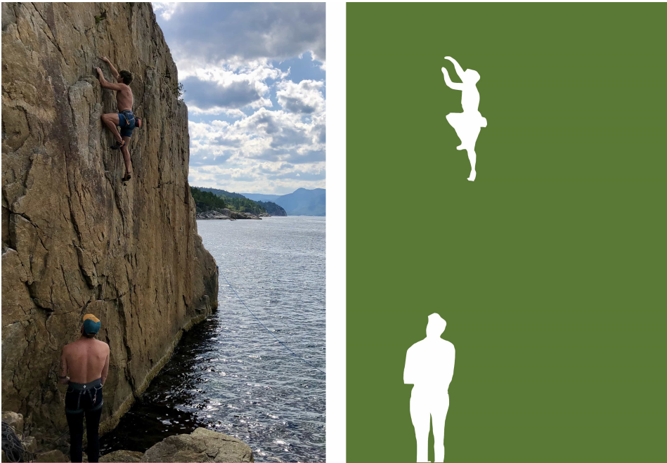
Figure 2.1: The first image shows two climbers on a cliff by the sea. The second image shows an image segmentation output based on the first image. In this case, the classes are people (white) and background (green).
