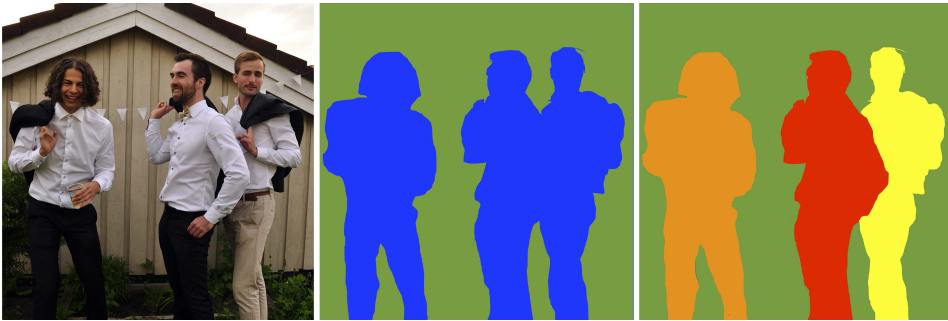
Figure 2.2: This figure illustrates the difference between semantic segmentation and instance segmentation. The leftmost image shows the original image. The middle image visualizes the result of a successful semantic segmentation. The people are all labeled with the correct class, but no distinction is made between the individuals. The rightmost image visualizes the result of a successful instance segmentation. All the people are correctly identified as individuals.
