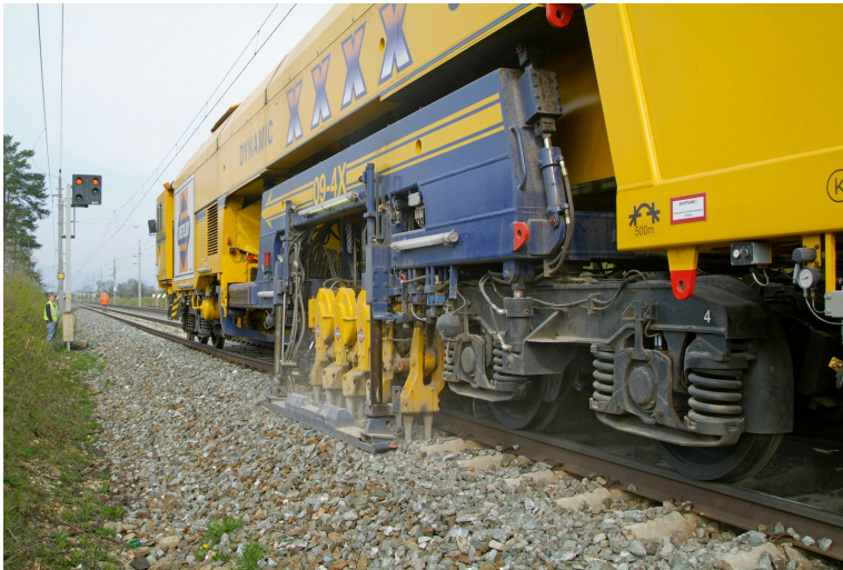
Figure 2.3: Tamping machine. ©Plasser and Theurer.
