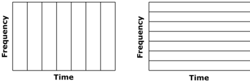
Figure 4.1: Generic picture of a time series analysis (left) and a Fourier analysis (right).
