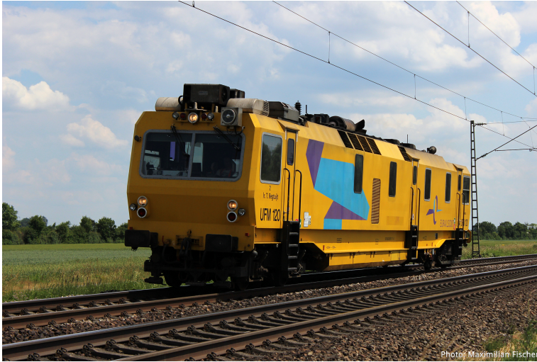
Figure 3.1: Track inspection car (TIC), the Eurailscout UFM 120. ©Fisher (2014).
