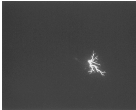
Figure 5: A partial discharge occurring along the interface between Nytro-impregnated pressboard and Nytro.
