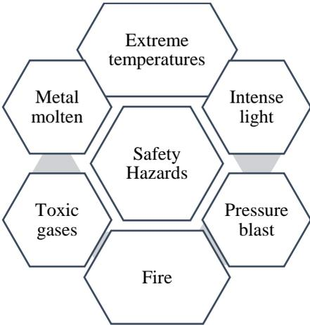
**Figure 2-2: Arc flash safety hazard [7]**
