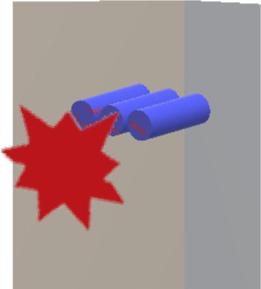
**Figure 3-2: Horizontal electrodes in a metal enclosure (HCB) reproduced after [1, 11]**
