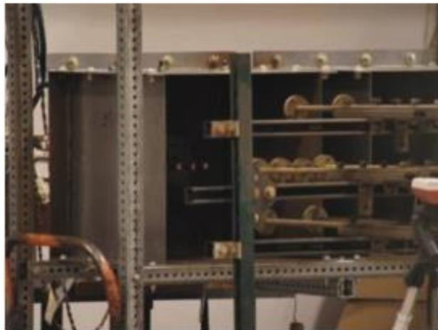
**Figure 1-5: HCB - Horizontal electrodes inside a metal enclosure [1]**
