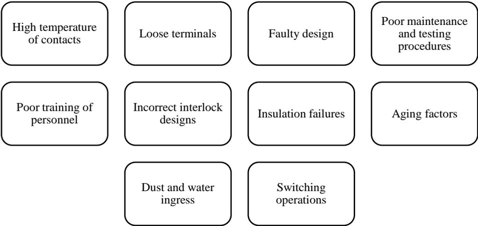
Figure 2-1: Example of arc causes [7]
