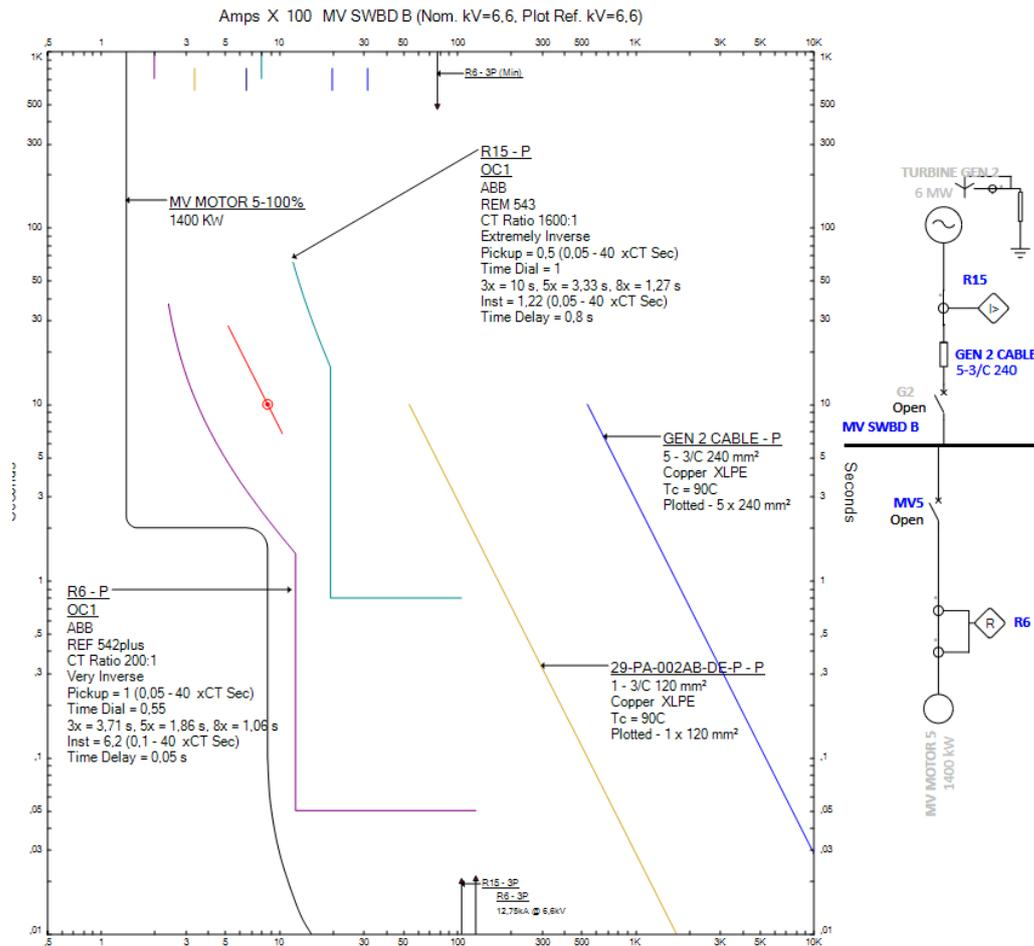
**Figure 1-7 Protection Coordination Curve**
