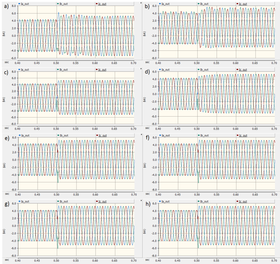
Figure 30: The current output of the inverter for different values of K_P and T_I during stable terminal voltage after fault initiation. The PI controllers are limited to [-1, 1] in all cases.
