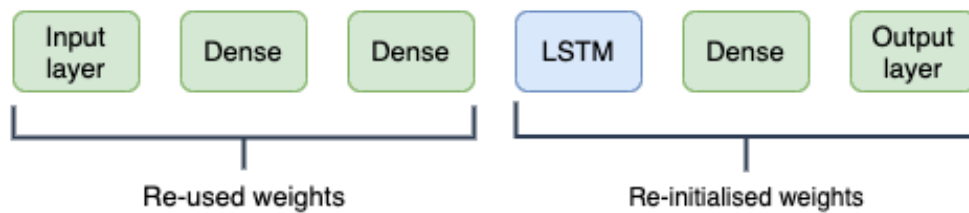
Figure 5.5: Architecture of TL model with the LSTM layer, layer five and output layer re-initialised
