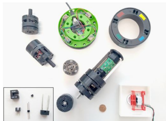
Figure 3.8: 3D printed low-cost force- and tactile sensing sensors. Courtesy of [20].
