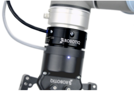
(a) 6-axis force-torque sensor mounted on a robotic wrist. Courtesy of [13]
