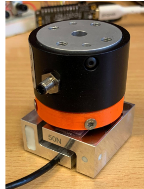
(b) The sensors fully assembled and locked together with LinkageType7
