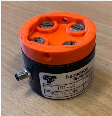
(a) The TRT-part mounted to the TRT-50 torque sensor
