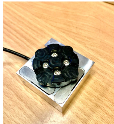
Figure 5.1: The K3D40 linkage-part mounted on the K3D40
