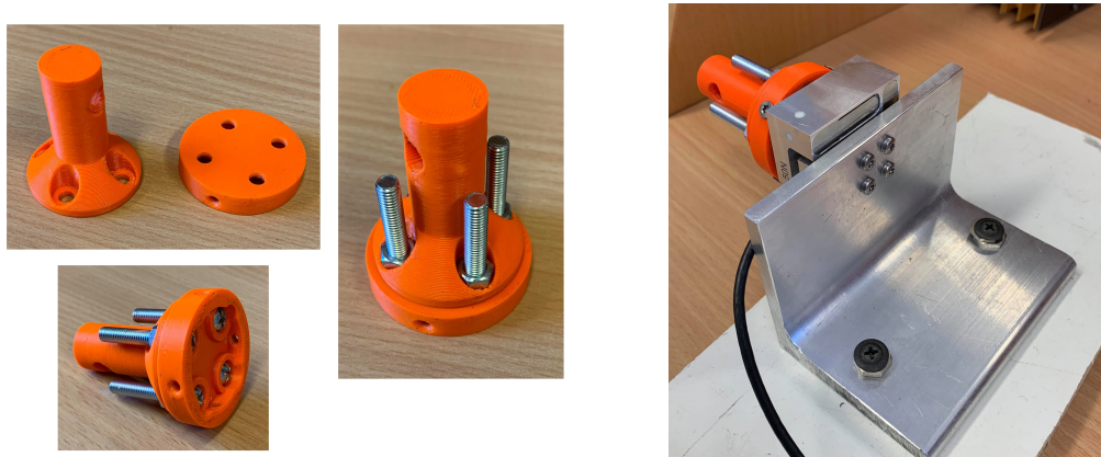
(a) Assembling the force-shaft for mounting, without a torque sensor (b) The force-sensor with the force-shaft, mounted to the test bench
