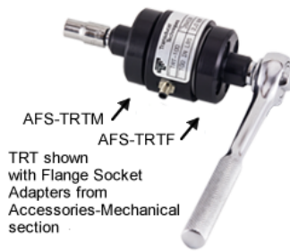
(a) Example of use with a TRT reaction torque sensor, in this example it's used to calibrate a manual wrench. Courtesy of [11]
