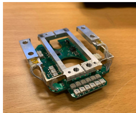
(b) The strain gauge sensor system (v3) mounted on the amplifier circuit board
