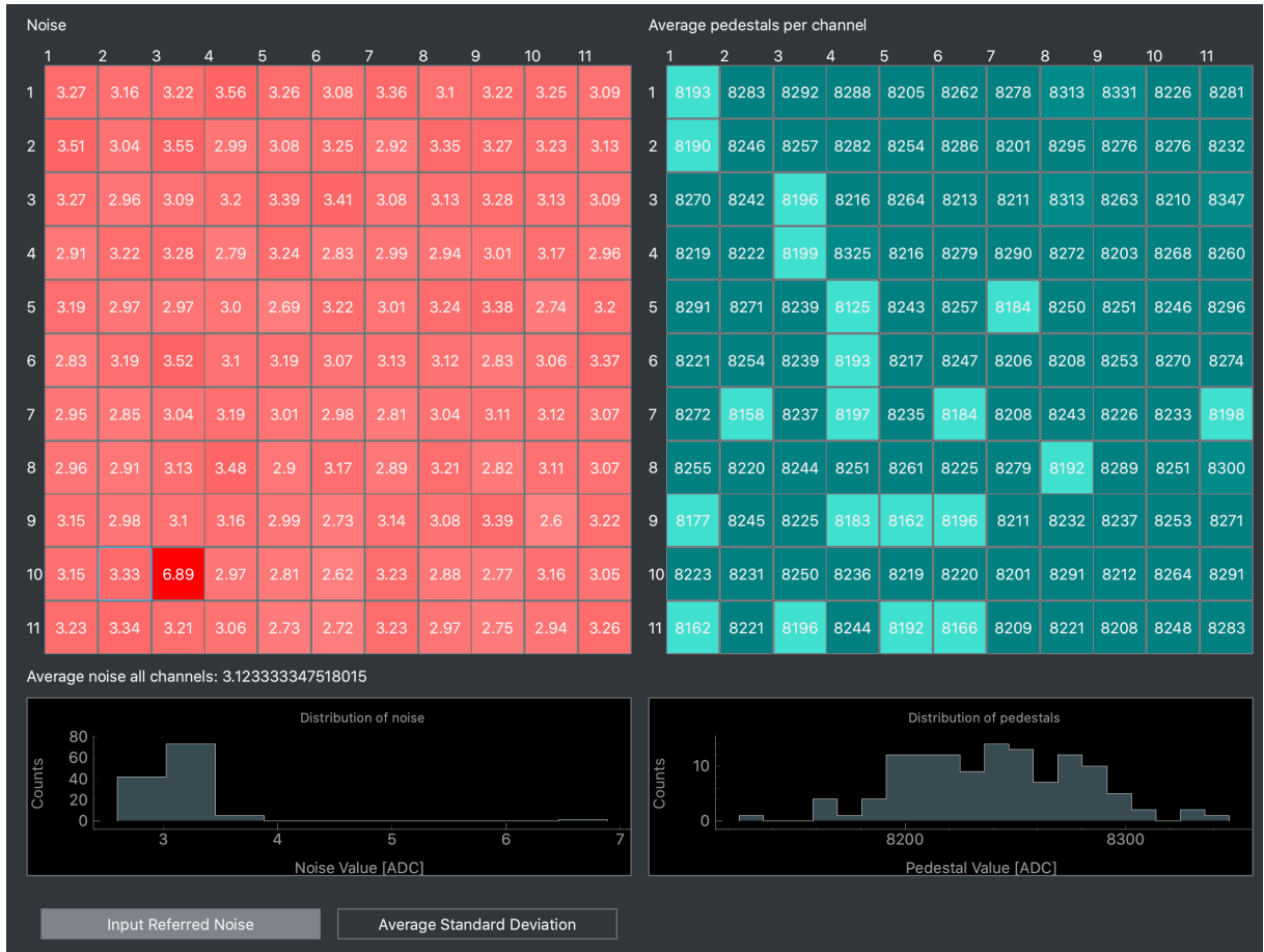
Figure 42 – Input referred noise and pedestal calculation from 1000 baseline readouts per channel. High voltage not connected.
