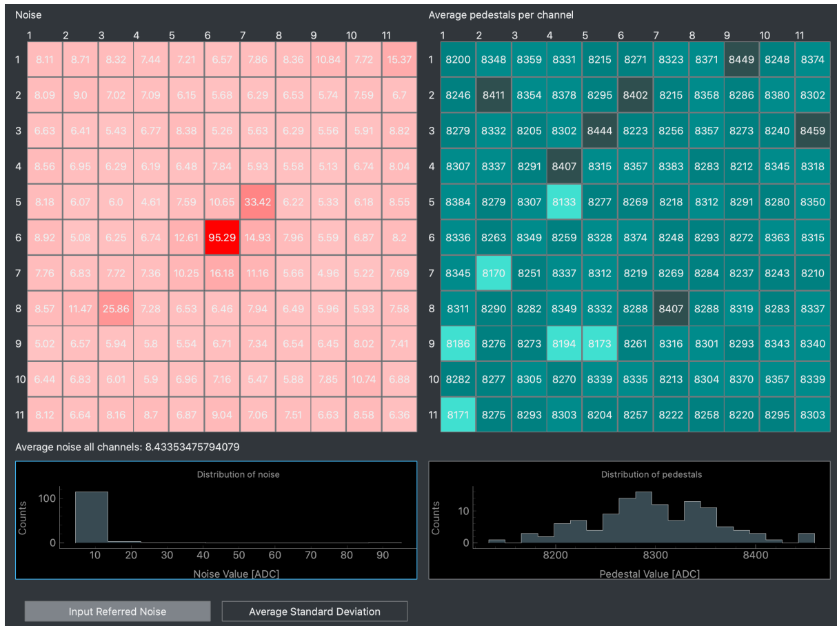
Figure 41 – Input referred noise and pedestal calculation from 1000 baseline readouts per channel. High voltage connected.
