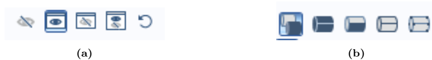
Figure B.2: Graphics Window toolbar in COMSOL Multiphysics. (a) Buttons to hide and restore objects. (b) Buttons to change selection of object types.
