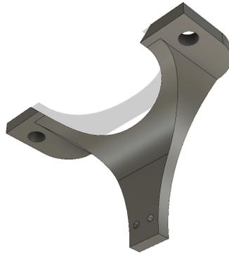
(a) Top limit switch holder, mounted on two M4 bolts underneath the stepper motor block
