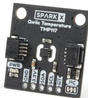
**Figure 3.5:** TMP117 temperature sensor mounted on a PCB module. Reproduced from [26].
