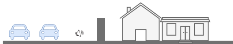
Figure 1.1: Illustration of a situation where a traffic noise barrier shields a neighborhood against traffic noise. The material of the barrier can be almost anything, but simulations to determine what provides for best airborne sound insulation is necessary.
