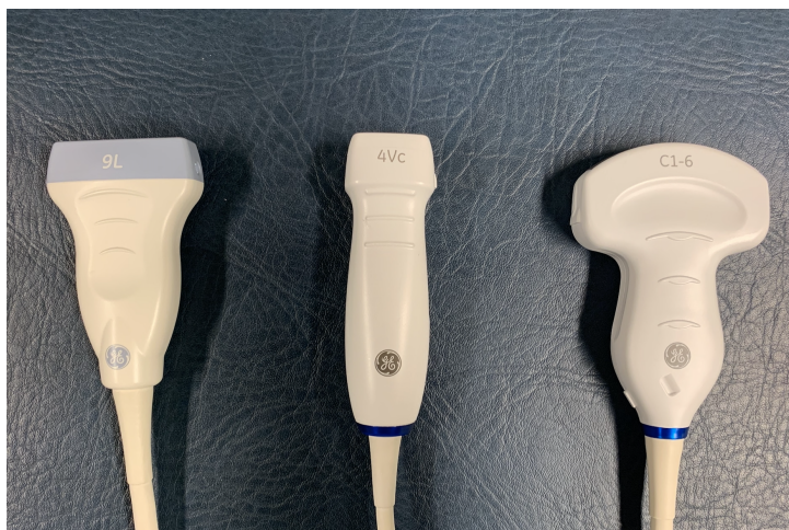
Figure 2.1: Linear array(left), phased array(centre) and curvilinear array(right)
