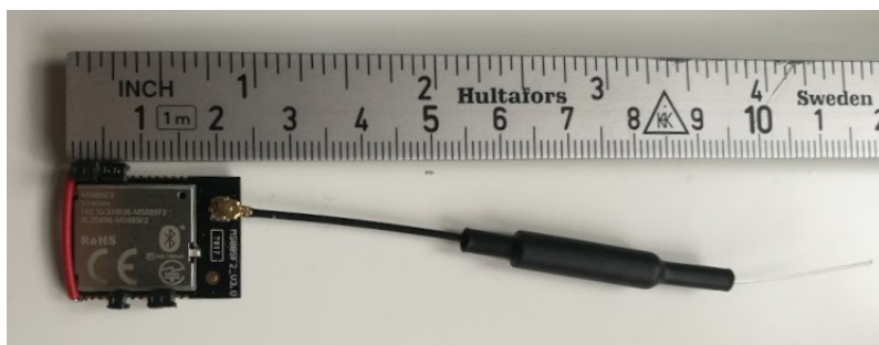
Figure 3.11: nRF module (MINEW MS88SF23) with connection headers and antenna attached.
