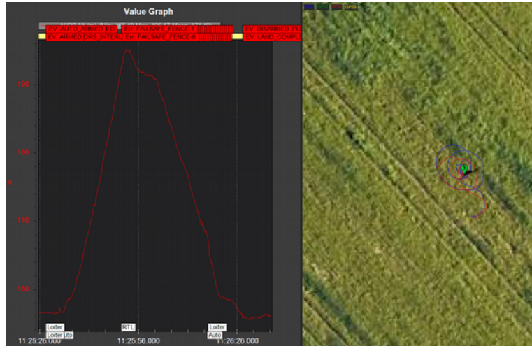
Figure 3.36: Altitude graph and event timeline around the Geofence failsafe triggering.
