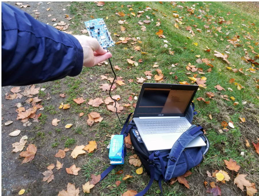
Figure 3.22: Development kit held manually at a height of 70cm. Connected to the computer for logging the results.
