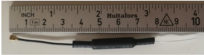
Figure 3.26: External 2.4GHz antenna with U.FL connector. Gain: 2.5dBi
