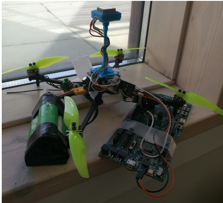
Figure 3.9: The UAV with a development kit connected over UART nRF52833 Development kit connected to the drone, powered by the drone and communicating over MAVLink over UART.
