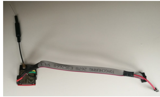
(b) Custom cable between MINEW MS88SF23 module and external programmer. For programming or debugging.
