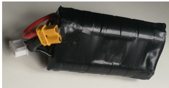
Figure 3.16: Sony VTC6 3S with a XT30 connector and JST balance charge connector. A spot welder was used to assemble the lithium-ion battery pack.
