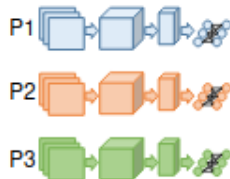
Figure 3: A visualization of the data parallelism architecture. The data is distributed among the different nodes in the compute cluster. The independent nature of SGD over mini-batches makes this technique highly scalable [5].
