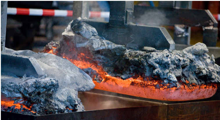
Figure 2.1: Carbon anode at the end of its life cycle.
