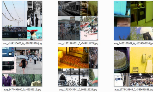
Figure 2.6: Mosaic data augmentation. Figure source: Bochkovskiy et al. [4].
