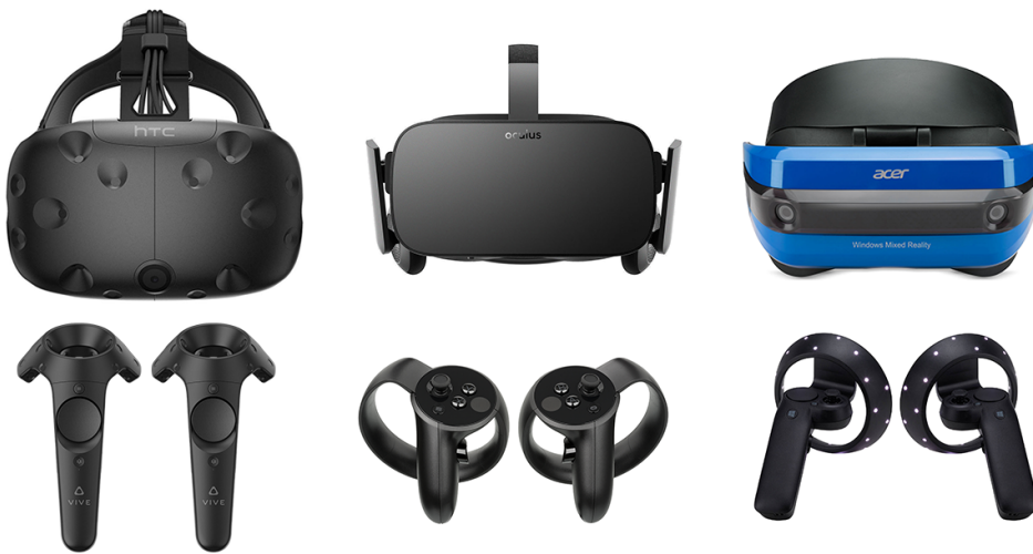
Figure 2.1: Three commercially available HMDs, Oculus Rift, HTC Vive and Acer Microsoft Mixed Reality headset.
