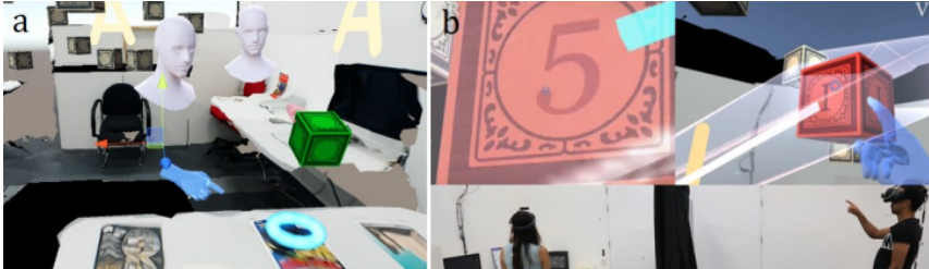
Figure 3.3: CoVAR in use with reconstructed environment (A left) and AR user (B left) and VR user (B right) looking at a block object. [33].
