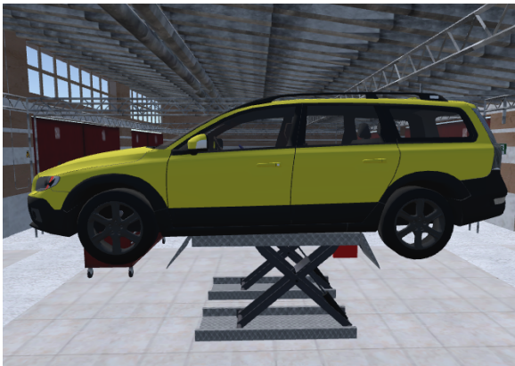
(a) The car lift mechanism in the application.
