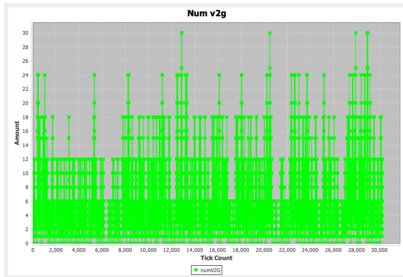
(a) Number of EVs involved in V2G charging throughout the tenth simulation of experiment 2.
