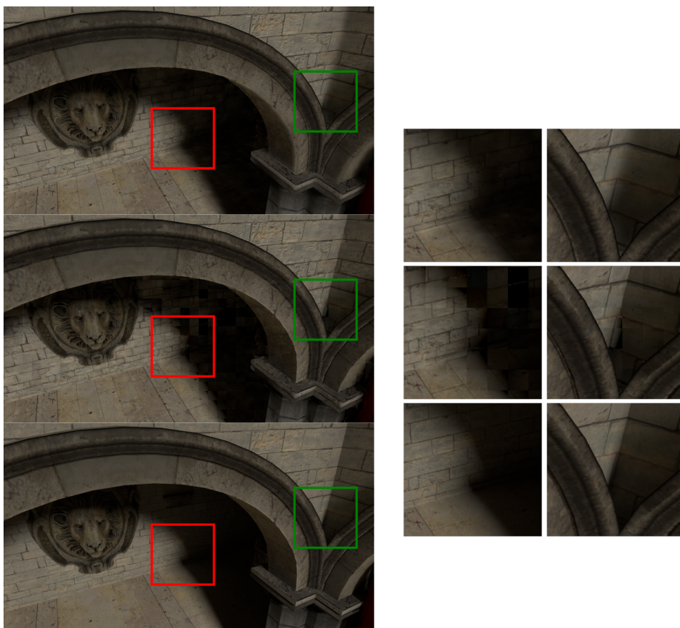
Figure 5.5: The first image from the scene Sponza. From top to bottom: SVGF, BMFR, Reference.
