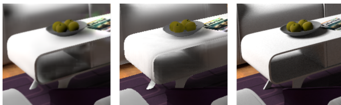
Figure 5.6: Detail from the last image of the Living Room image sequence. From left to right: BMFR, SVGF and Reference. The table has been within field of view for about 30 frames. BMFR still shows off significant amounts of artifacts, while SVGF has converged at a slightly inaccurate but closer lightsetting.
