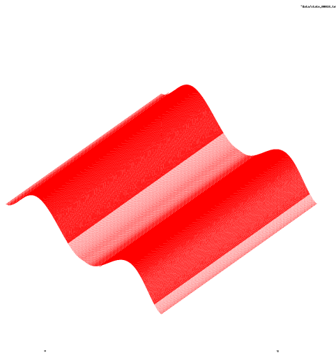
Figure 7.4: Wave from middle after being split and moving outwards. The refined areas have a higher density of points.
