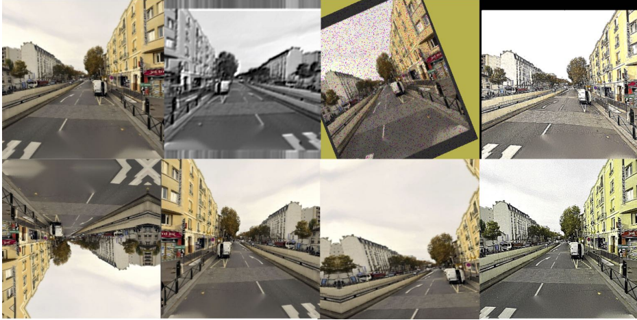
Figure 3.4: Perception data augmentations. A set of randomly generated augmentations from a single image from the Mapillary dataset. Each image includes several different augmentation of different magnitudes. Some of the obvious augmentations ordered from top left are: greyscale (second image), rotation (third image), mirroring (sixth image) and hue/saturation changes (eight image). The top left image is the original.
