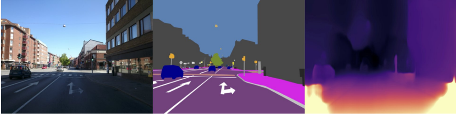
Figure 3.2: Sample from the Mapillary Vistas dataset. A selected image from the Mapillary training data. It shows the original image to the left and the labeled segmentation in the center. The right-most image is a depth map generated by Monodepth2.
