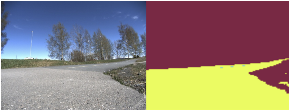
Figure 4.9: Real-world driving data. A visualization of a road without lane lines. The left image is the original image from the vehicle’s camera, while the right image is the resulting segmentation after processing by the perception model. Yellow is categorized as road, blue is lane lines and red is unlabeled.
