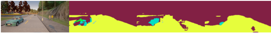
Figure 4.1: Images segmentation samples. This image shows an original image from CARLA, with segmentation maps generated by ResNet50-SegNet, MobileNet-SegNet and VanillaCNN-SegNet in order from left to right. Note that the models were trained on real-world data and therefore have never seen a simulated environment.
