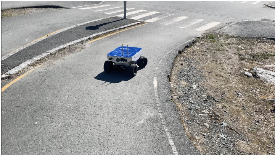
Figure 4.7: SPURV Research vehicle during evaluation. An image of the SPURV Research vehicle while driving on our test track. The driving environment is a downscaled urban environment with intersections and traffic lights.
