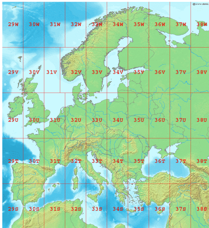
Figure 6.2: Illustration of UTM zones. "LA2-Europe-UTM-zones.png". Image is public domain. No changes made. https://upload.wikimedia.org/wikipedia/commons/9/9e/LA2-Europe-UTM-zones.png .
