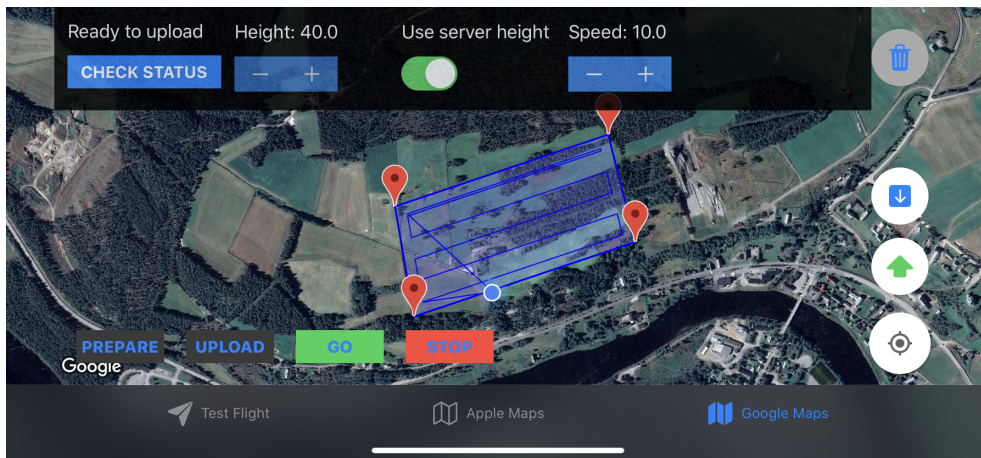
Figure 8.6: Area and path covered in test at 40 meters altitude.
