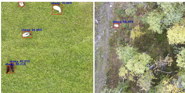
Figure 5.2: The left image showing the good contrast the green grass gives, while the right show a false positive with a white stone.
