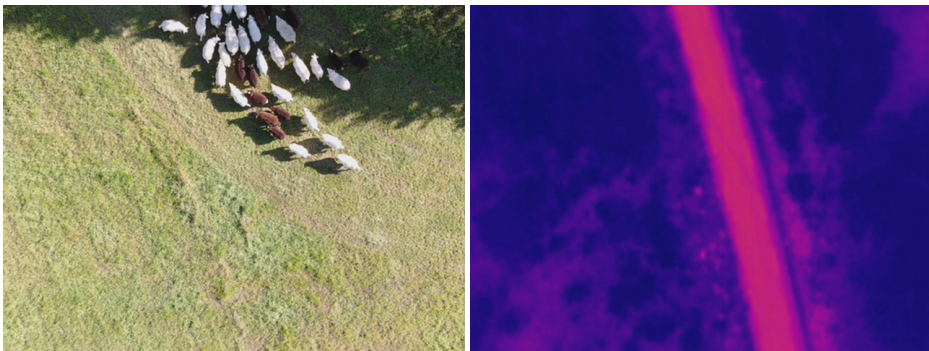
Figure 4.3: Examples of unusable infrared images, The left image was in the location of an infrared image and has a resolution of 640x480 making it unusable for both the infrared and RGB network. Image on the right used a different color palette than gray scale.
