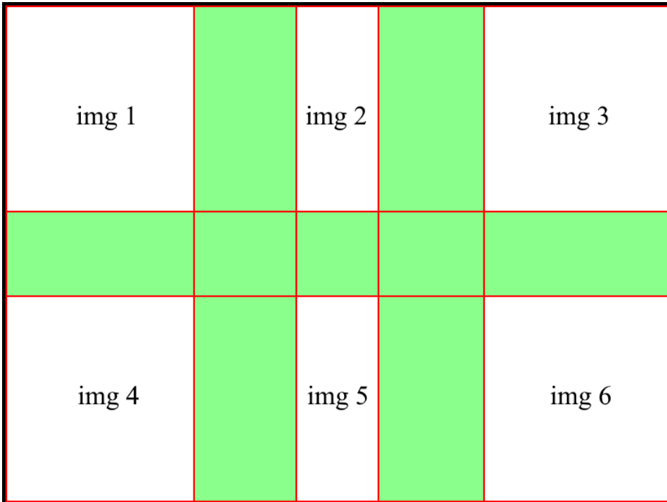
Figure 5.1: Illustration of the splitting process. The original image is split into multiple, smaller images. The overlapping areas are marked green.
