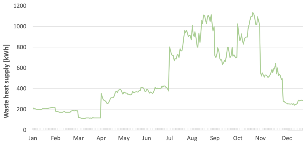
Figure 6.4: Hourly averaged local waste heat supply at Leangen. Source: SINTEF Energy Research.
