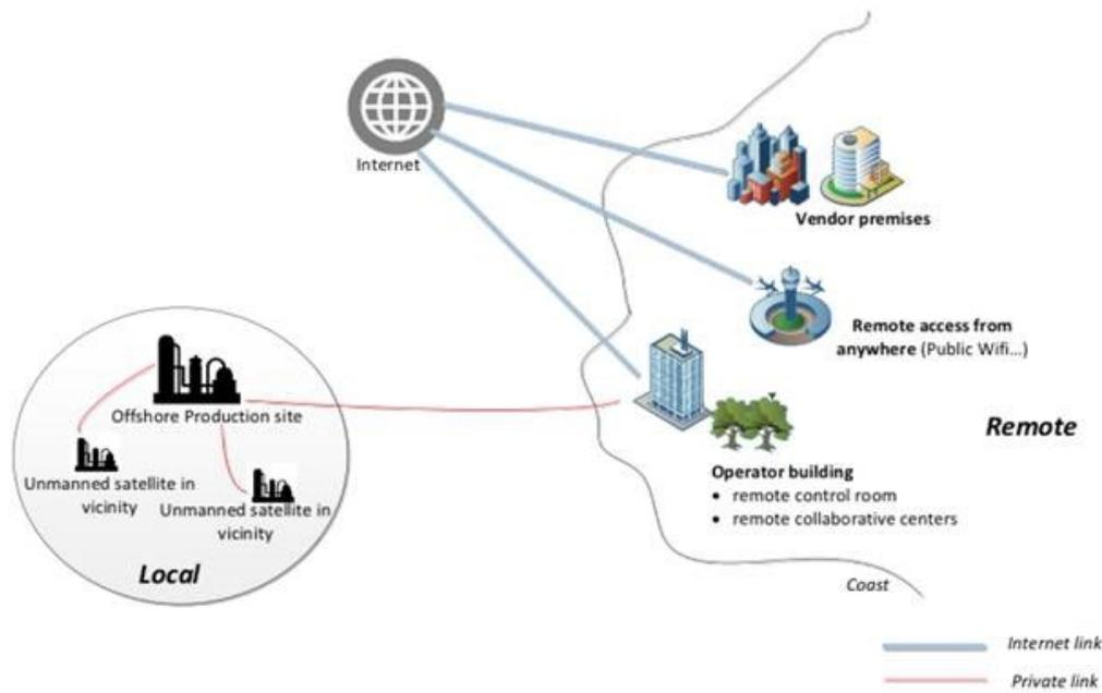
**Figure 2.3:** The ecosystem for remote operation in Oil and Gas
