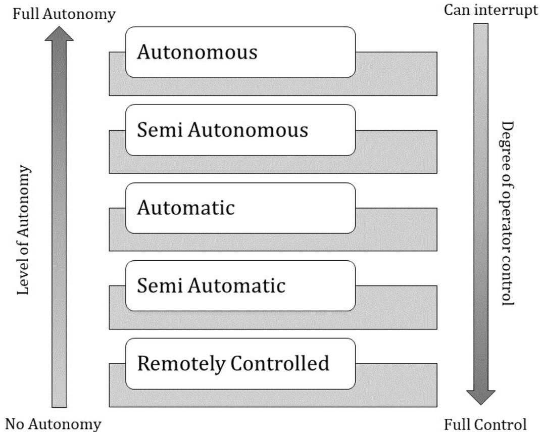
**Figure 2.1:** Level of Autonomy and degree of operator control
