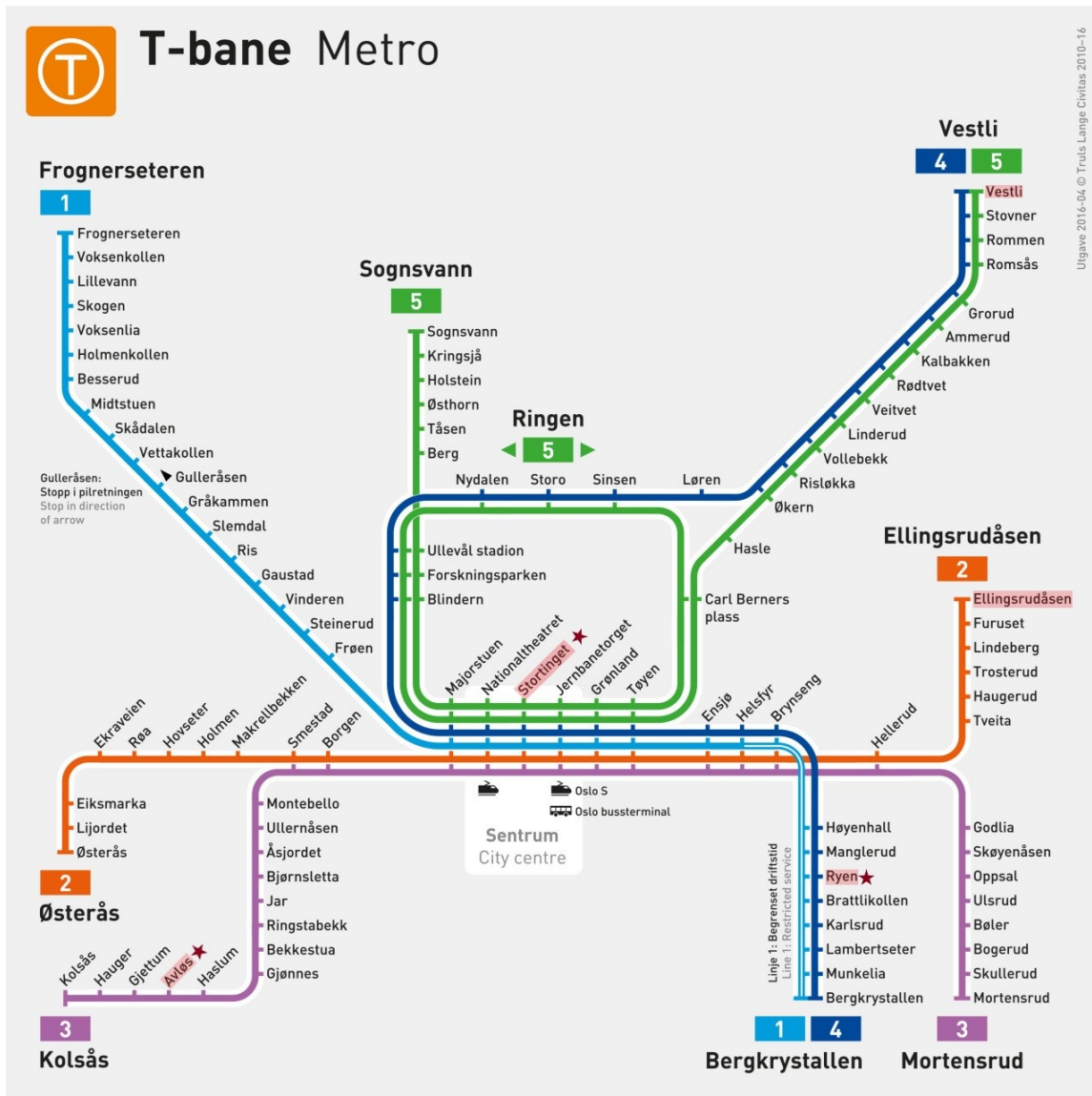
Figure 2.2 – The Oslo Metro schematic map. The stations with a co-located depot are marked in red. Names marked with a red star are the associated stations where depots have cleaning equipment. Copyright Truls Lange Civitas
