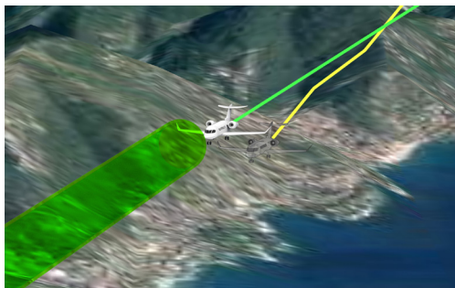
Figure 3.46. The green curve shows trail of the reference data, the yellow curve shows the trail of the nav data.
