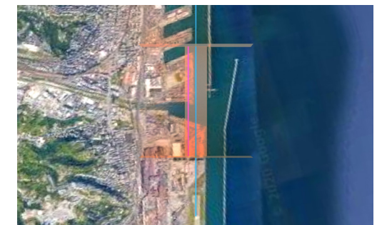
Figure 3.66. The alignment of localizer is a horizontal offset of the ideal path.
