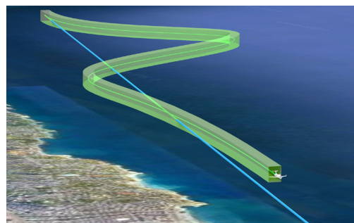
Figure 3.49. The tunnel should be drawn along the reference path and shows the tolerance.
