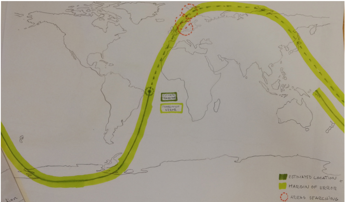
The wall mounted screen #1 shows the simulated trajectory of the satellite's orbit before any contact is made. The circles near Norway on the map are where the ground station radio signals are searching for the satellite.
