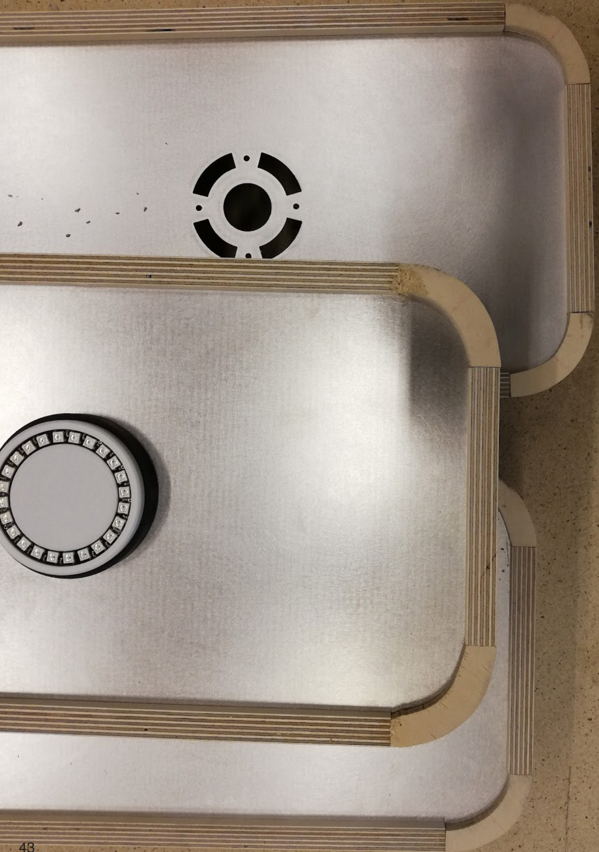
Figure 5.8. Game poles with aluminium face and wooden frame, with assembled button.
