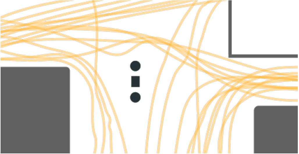
Figure 5.7. Traffic mapping of installation area.
