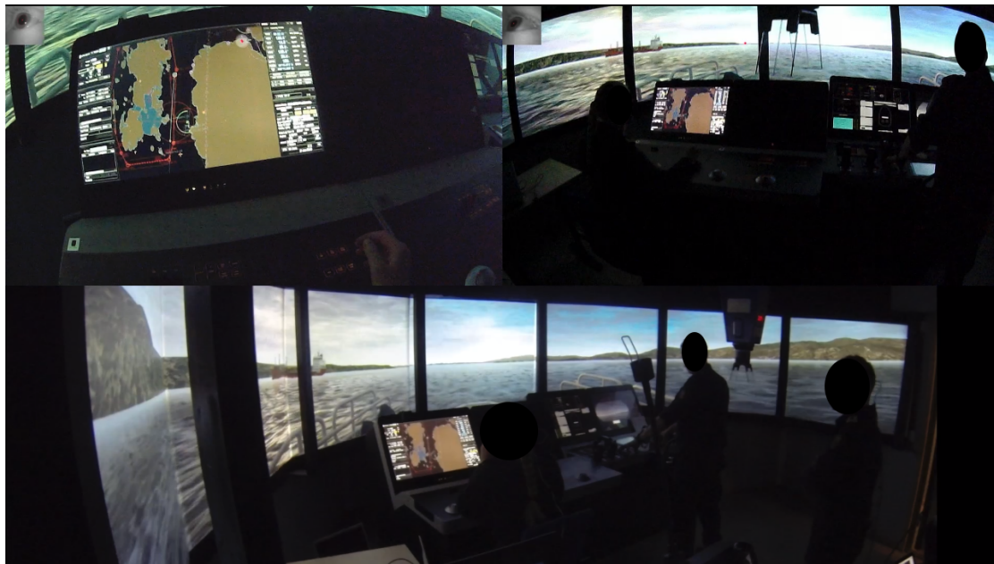
Figure 4: Assemble: Up = Eye-tracker incl. eye(R) + gaze-point (Left - Assistant; Right - Navigator); Below = scene camera (GoPro)
