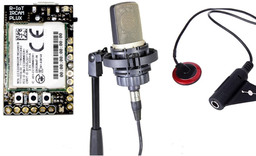
Figure 3.1: Left to right: BITalino R-IoT, condenser microphone, contact microphone
