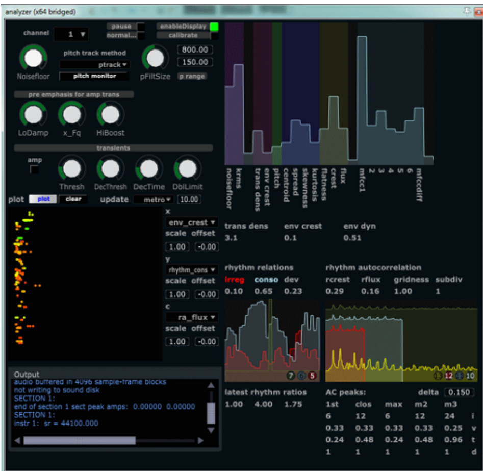
Figure 4.1: Brandtsegg's analyzer VST offers a lot of control over the input signal.
