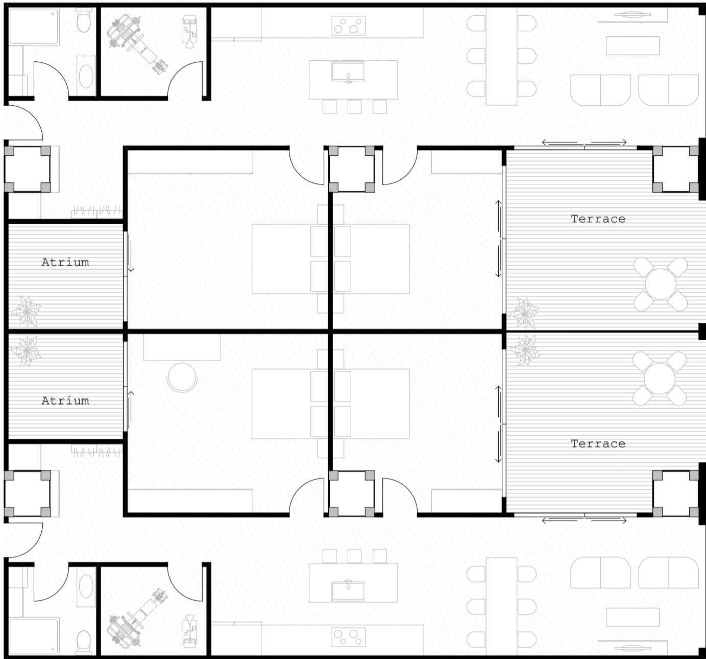
Figure 19. Terrace apartment floor plan 1:100
